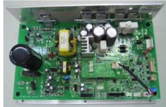
LCB with the transfer board (Part number # 1000336916 )
