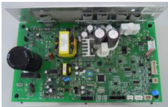
LCB without the transfer board (Part number # 1000203336 )
